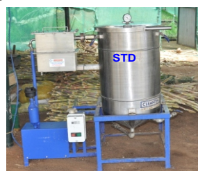
Sett Treatment Device (STD) to treat sugarcane setts
